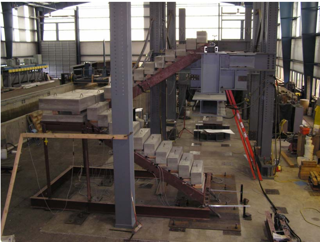
Fig. 8 – Specimen loaded with blocks simulating full factored design gravity load per Eq. 2 (blocks stacked on top of one another).
